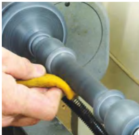
▲ Pic.35 With the lathe running slowly, use a piece of Nyweb pad equivalent to '0000' wire wool to finish of the liming process. I like to apply fairly hard pressure to get the desired effect before applying a couple of coats of clear gloss lacquer
